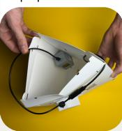
Fold and attach the delta trap's back edges.
