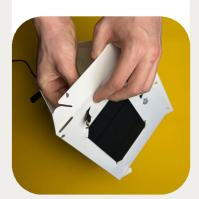
Connect the solar panel's cable with the shorter cable coming out from the battery.
